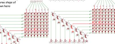
Power is a significant driving force in this circuit design. You may wonder why we need all those transistors to provide current paths to ground for the rows - can't we just connect them directly to the microcontroller? Well, if all the LED's in a row were on then over 100mA of current would be surging through the transistors which are rated for 600mA, while the microcontroller pins are rated for 20mA.
